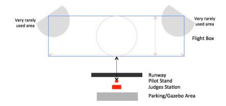
Dedicated runways will be prepared for the event. They will be made of approximately 300X30 mt cured grass. They will provide access to an airbox of approximately 800X300 meters. The average distance between the pilot stand and the front display of the flight box will be approximately 150 meters. Therefore, the pilot will be able to perform rolling circles that will
